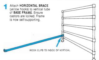
Attach spare end of brace to end of other BASE FRAME. Attach 2nd HORIZONTAL BRACE (yellow hooks) to other side of frame. Attach PLAN BRACE(S) (black hooks) diagonally onto the vertical tube below the lowest base frame rung, or as low down as possible.
