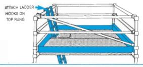
LADDER "CHANGE-OVER" PLATFORMS: One WALK-THROUGH PLATFORM is required to enable safe ladder change-over on towers with more than one ladder. Attach platform before ladder
