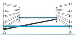
Attach four **DIAGONAL BRACES** to the base of the unit as shown. Level the unit using the adjustable legs. The base is now complete.
