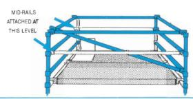
To complete the WORK PLATFORM, first fit the TOEBOARD to allow the trap-door on the platform to open freely. Finally attach the LADDER through the ACCESS PLATFORM, as shown, and clip on stand-off hooks, at base of ladder, to the corresponding rung on the frame. Ensure the access door movement is not impaired.
