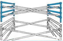
Fit the PLAIN PLATFORM first, then the WALKTHROUGH PLATFORM with the hinges of trapdoor to the outside of tower.
